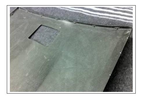
The final step is to enlarge the oil door hole as needed for your type of oil door and hinge. Make sure that the hole is big enough in order for the oil door hinge and fasteners not to interfere.
