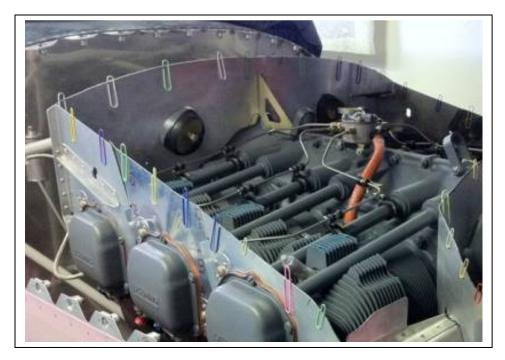
The flanges of the plenum can be protected at this stage by applying strips of UHVM tape to it. Also remove the angle bracket between the top center of the engine and the rear baffle plate as it might interfere with the plenum fit.
