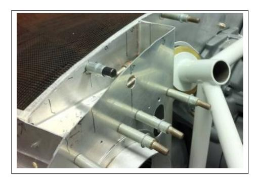
Test fit the top cowl and have a careful look at where the front ends of the plenum interferes with the top cowl inlet air ramps. The front ends are slightly longer than
