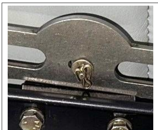
Figure 2: Clevis pin with cotter pin
